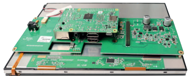
Compact and secure assembly of TFT-module and Raspberry Pi 3
